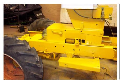
This kit is easiest if the rear fenders and electric lift are off. This is a good time to change the hytran fluid, reseal the rear plate on the differential and any other general work. If you have a hitch on back, remove it and replace the bolts with (3) bolts that are <sup>1</sup>/<sub>4</sub>" shorter.
