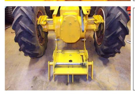
Attach the 3 point plate to the previously installed brackets with the supplied 7/16" bolts, nuts and lock washers. Do not tighten yet – finger tight only.
