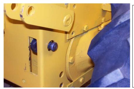
Rotate the plate up into position and put the link shaft thru the inner ears and align everything so that you can insert the 5/8" pin thru the hole, ears and shaft. Secure the pin with a cotter pin.
