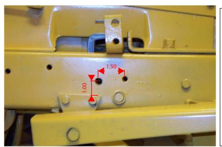
Using a measuring device, measure up 1" from the foot rest bracket and 1 ½" back from the hole shown.
