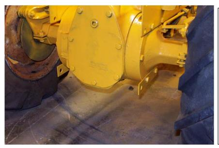
Attach the rear brackets to the axle housings by taking out the existing lower 2 bolts and putting the bracket over them and re-inserting them.
