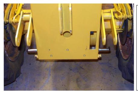
Attach the 3 point pins to the plate using the supplied nuts and lock washers. Best is if you can keep the holes straight up and down. Tighten securely. The plate has 2 sets of holes for the pins. The bottom is considered "Stock", but if you need a different lift configuration due to equipment needs, you can move them to the upper holes.
