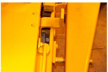
Slide the shaft up to meet the bolt that you inserted earlier. Push the bolt thru now and secure with the supplied nylon lock nut. There is not a lot of room to work, and a 3<sup>rd</sup> hand can come in handy. Tighten the nut snugly and then back off ½ turn to allow rotation and eliminate binding.
